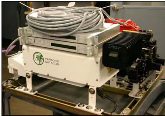
125W Ku-Band 1:1 Phase Combined SSPB System with FPRC-1100 Controller and RCP2-1100 Controller for L-Band redundancy
