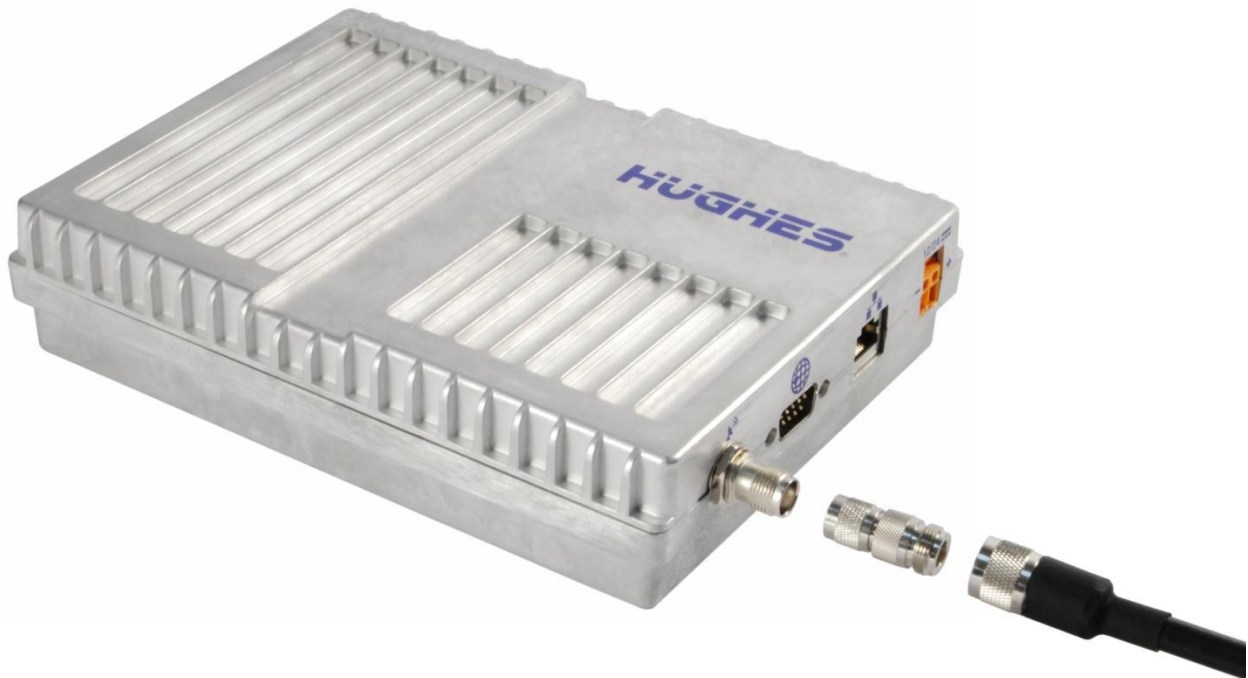
Figure 21 – Connect cable to TNC connector on IDU
